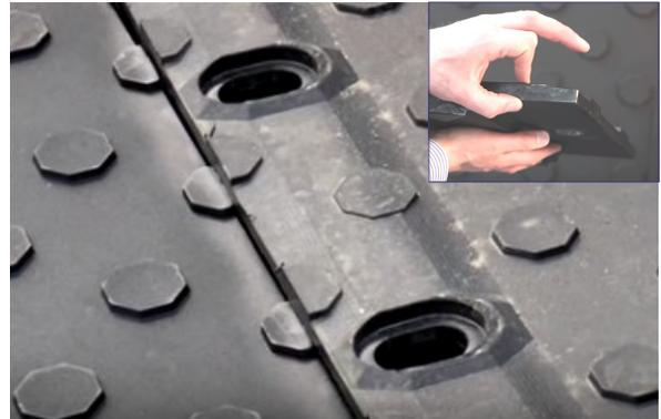
2. MaxiTrack mats are connected via the overlapping flange joints (see inset top right). The slotted holes allow for expansion and contraction.
