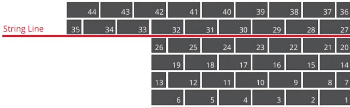
**String Line** *Order of installation for car parks and pad areas, working uphill from the bottom of the slope*
